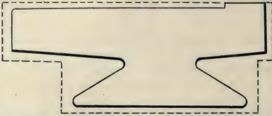
FIG. 119.—Outline of Commutator Segment.
